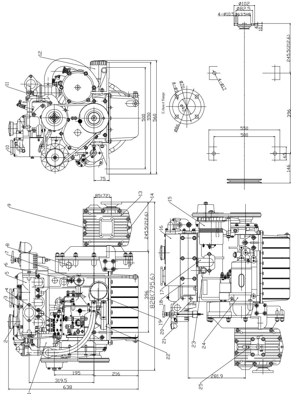
Note: The dimension in bracket is only for matching ZF12M gearbox.
